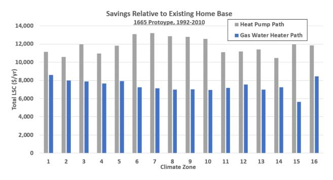
Figure 15. Heat pump water path compared to gas with solar thermal.
